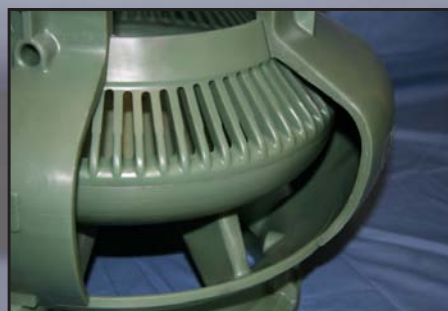
The complex grid is vital to the functioning of the part. The casting is injected in three waxes and poured in one shot.
