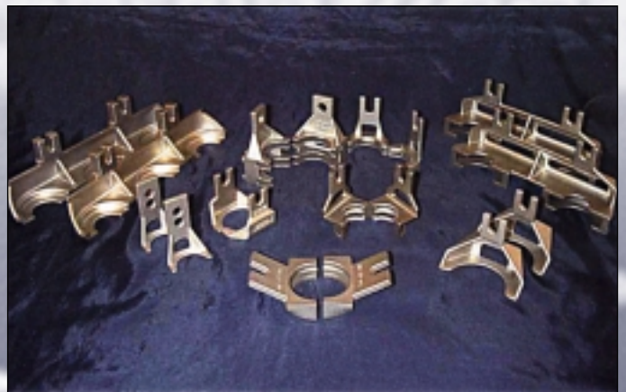
Single, double and triple gob take out castings. - Photo by Roger Schultz
