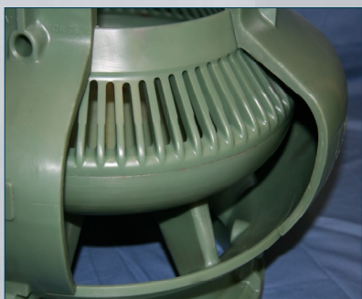
Cross section of 3 Piece Wax Assembly
