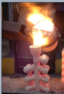
Recyclable Ceramic Shells Shape the Liquid Metal
